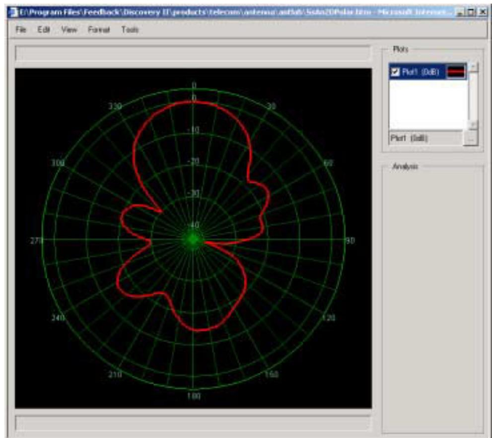
Figure 2-1-3: A Typical Polar Plot
