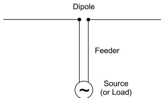
Figure 2-2-1: A dipole and feeder
