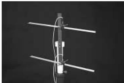
Figure 2-4-6: Dipole Stacking
