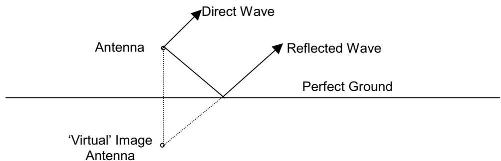
Figure 2-6-1: Reflected and Incident Waves
