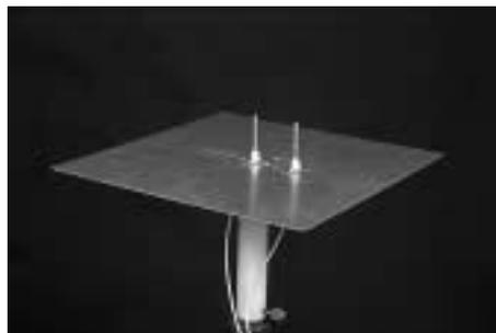
Figure 2-8-1: Two Monopole Assembly on Tower
