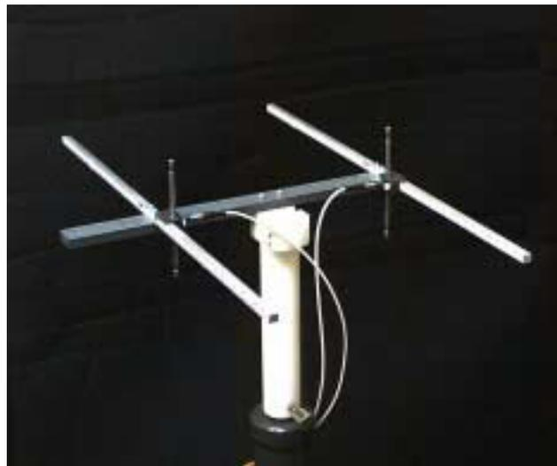
Figure 2-4-7: Dipoles for Elevation Plot
