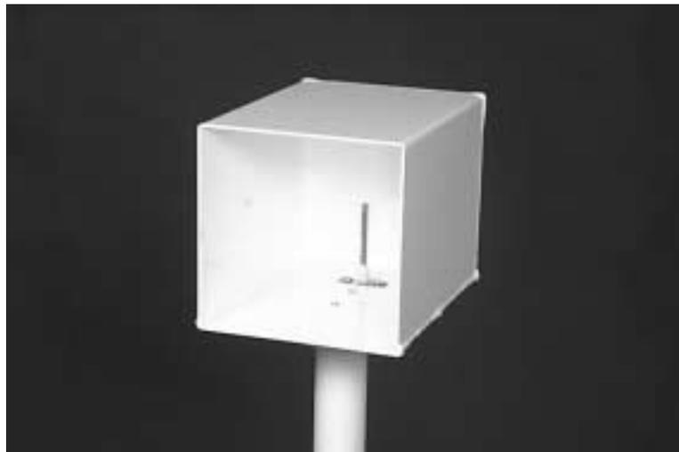
Figure 2-14-1: Horn assembly
