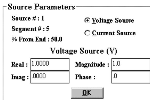
Figure 2-4-4: Source Parameters Set-up Dialogue Box
