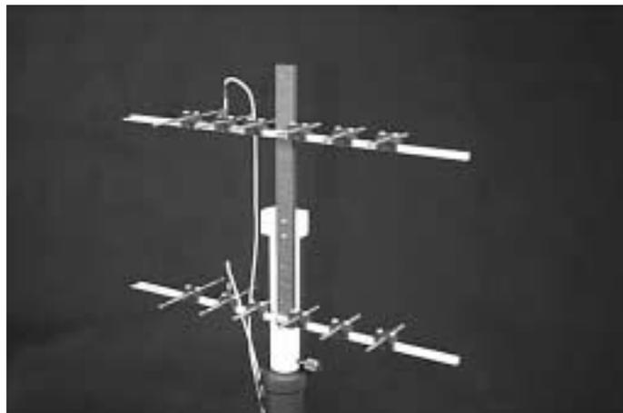
Figure 2-13-2: Stacked yagi assembly
